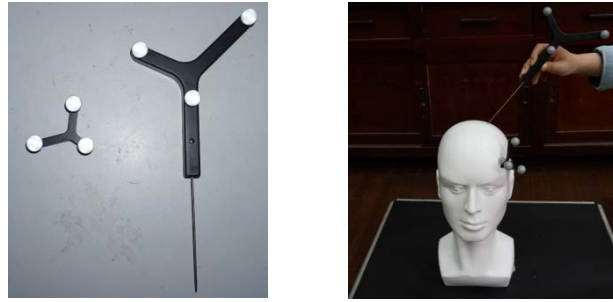
(a) Instrument and trackers design. (b) Puncture operation.
